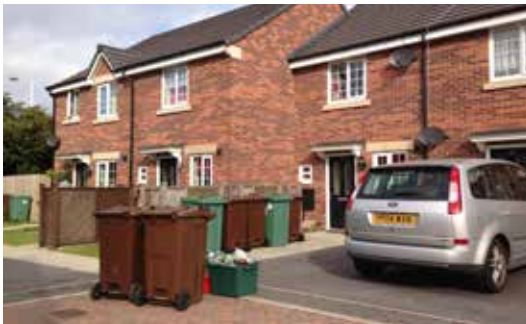
Figure 5 West Yorkshire example. Bins are wheeled to the shared surface on collection days without a dedicated area for them to stand
